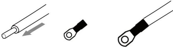
Step 2: Connect the power grid cable to the terminal shown in the figure below, and use a screwdriver to fix and tighten the cable.
