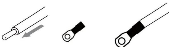
Step 2: Connect the load cable to the terminal shown in the figure below of the inverter, and attach it firmly with a screwdriver.
